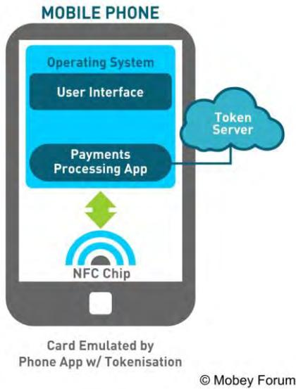
Figure 4: Card Emulation by Phone Application Solution
