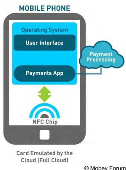
**Figure 2: Full Cloud Based HCE Solution**
